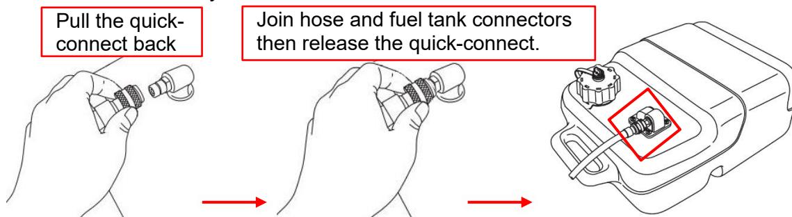
4. External Fuel Tank is connected.
