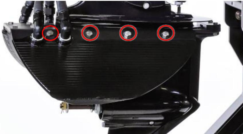
9. Manually tip the fin over the basin until all coolant is drained.
